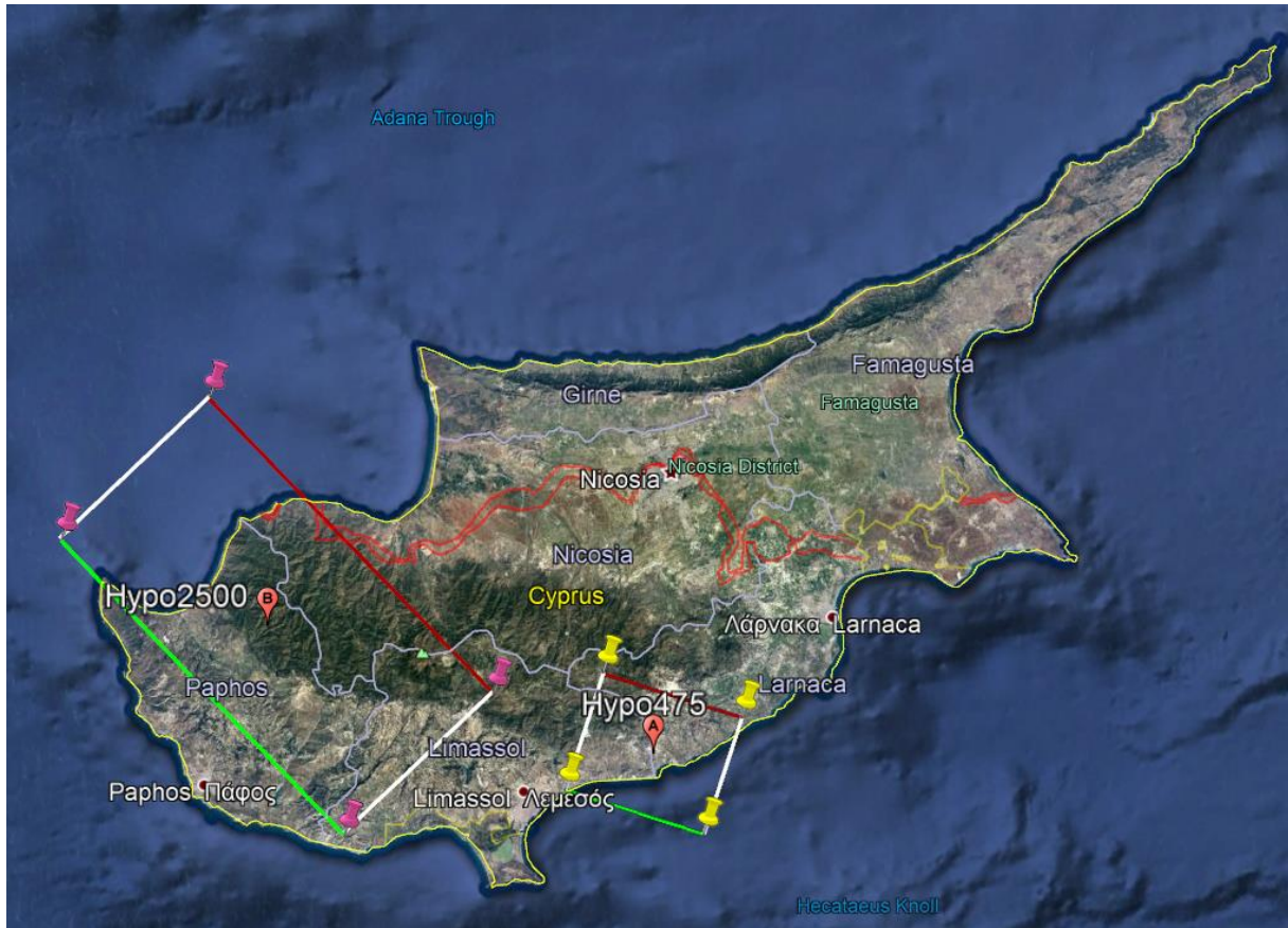
Figure 4.29. Projected geometry of faults of seismic scenarios on the island of Cyprus (green line depicts top edge of the fault plane, red line bottom edge)
