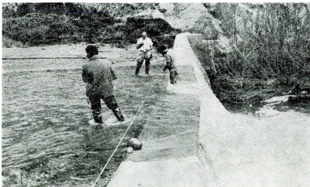
Current meter measurement for the calibration of the measuring weir at Phinikaria flow gauging station on Yermasoyia River. WDD Photo 48EN-15A (6.3.80).
